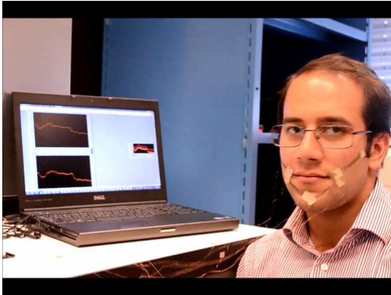
“Tunable high-stretch metal sensor” Firouzeh & Paik (2015) ME-410 Mechanical Product Design & Development
